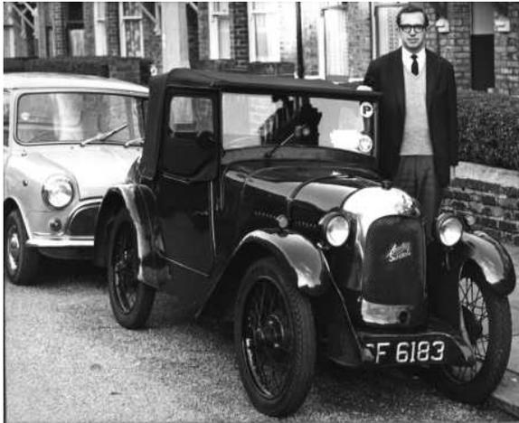
A hood frame and side screen frames were made from mild steel concrete reinforcing rod. A new hood and tonneau were made in Slades Hill, Enfield. The car shared the workshops with a large fabric Bentley which was being recovered and an early Austin Seven Chummy which was having a tailored dust cover made (at twice the price of my hood and tonneau). I was very pleased with the hood but the tonneau was not such a success as it did not fit easily over the hood frame when folded down.
